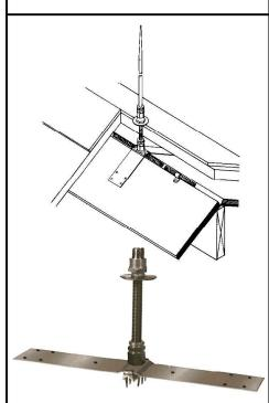
NO. 71C-A CONCEALED RIDGE SADDLE ASSEMBLY USED ON NEW CONSTRUCTION WHERE ROOF SADDLE AND CONDUCTORS CAN BE CONCEALED. TYPICALLY USED WITH CEMENT, CLAY TILE, OR SLATE ROOFS, OR WHERE LOW PROFILE VENTS ARE USED AT ROOF RIDGES. THIS ASSEMBLY COMES COM-PLETE WITH A BASE ADAPTER, 41/2" LONG, THREADED RISER, LEAD SEALING WASHER, AND EXTERNAL ADAPTER TO FIT ALL ADAPTER TYPE AIR TERMINALS FOR CABLES THROUGH NO. 506
