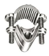
**NO. 240**—THIS CAST BRONZE PIPE CLAMP IS TIN COATED TO PREVENT CORROSION. CLAMP ACCEPTS CABLES THROUGH NO. 506 AND PIPE OR TUBE DIAMETERS UP TO  $1\frac{1}{4}$ " 0.D. USED FOR BONDING MAIN SIZE CONDUCTORS TO MAIN WATER SERVICE PIPING OR ELECTRICAL CONDUITS, ETC.
