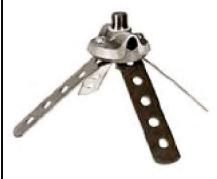
NO. 79-A FOUR LEG ADJUSTABLE BASE FOR MOUNTING AT CONE-SHAPE OR ROUNDED VENTS OR MECHANICAL EQUIPMENT, ETC. CAST BRONZE CABLE CLAMP IS FOR ALL ADAPTER TYPE AIR TERMINALS AND FITS CABLES THROUGH NO. 506.
