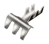
NO. 128-A STAMPED BIMETAL TEE SPLICER FABRICATED FROM A SPE-CIAL "ALCO PLATE" MATERIAL FOR JOINING A MAIN SIZE ALUMINUM TAP CABLE THROUGH NO. A37 TO A MAIN SIZE COPPER RUN CABLE THROUGH NO. 506.
