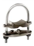
**NO. 802**–A U-BOLT TYPE PIPE BONDING CLAMP WITH A CAST BRONZE CABLE CONNECTION AND 5/16" STAINLESS STEEL U-BOLT. THIS CLAMP ACCEPTS ALL CABLES THROUGH NO. 507 AND A MAXIMUM PIPE O.D. OF 17/16".
