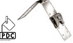
NO. 71X-A 2" WIDE COPPER SADDLE WITH A PREMI-UM DIE CAST BOLT PRESSURE CABLE CLAMP FOR CABLES THROUGH NO. 506. STUD ACCEPTS ALL ADAPTER TYPE AIR TERMINALS, SADDLE CAN BE FIELD ADJUSTED TO ALL ROOF PITCHES.
