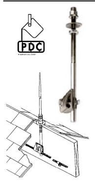
NO. 24-A THROUGH ROOF BASE FOR CONCEALED MOUNTING AT ROOF RIDGE LOCATIONS. ASSEMBLY INCLUDES AN ALL THREAD 3/6" X 12" LONG RISER BAR, CAST BRONZE CABLE CLAMP FOR CONDUCTORS THROUGH NO. 506, LEAD WASHER FOR WEATHER SEAL ABOVE THE ROOF, HEX NUT, AND FLAT WASHER TO SECURE RISER BELOW THE ROOF, AND NO. 28 ADAPTER TO ACCEPT ALL ADAPTER TYPE AIR TERMINALS.
