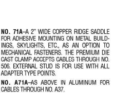
NO. A71A-AS ABOVE IN ALUMINUM FOR CABLES THROUGH NO. A37.
