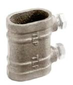
**NO. 519—**A VERY LARGE, HEAVY DUTY 2%" LONG CAST BRONZE GROUND ROD CLAMP FOR 34%" GROUND RODS. THIS CLAMP HAS TWO 546% STAINLESS STEEL SET SCREWS AND WILL ACCEPT CABLES THROUGH NO. 507.
