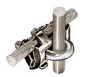
**NO. 493**—THIS  $\frac{5}{16}$ " STAINLESS STEEL U-BOLT TYPE ROD TO CABLE CLAMP IS A VERY VERSATILE CONNECTOR FOR CLAMPING ALL MAIN SIZE CABLES FROM NO. 29X THROUGH NO. 507 TO GROUND RODS THROUGH  $\frac{3}{4}$ " DIAMETER. THIS CLAMP CAN ALSO BE USED TO CONNECT AIR TERMINALS, RISER BARS, REINFORCING RODS OR SMALL PIPING (THROUGH  $\frac{7}{8}$ " DIAMETER) TO CABLES.
