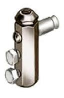
NO. 90-A MACHINED BRASS CONNECTOR FOR %" AIR TERMINALS. INTENDED FOR VERTICAL MOUNTING OF %" "LESS ADAPTER" TYPE AIR TERMINALS AND INCLUDES A STAINLESS STEEL MOUNTING BOLT AND LEAD EXPANSION ANCHOR. BASE REQUIRES ADDITIONAL SUPPORT ON THE AIR TERMINAL TO INSURE ADEQUATE SUPPORT.
