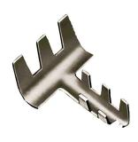
NO. 120-A SOLID COPPER TEE SPLICER OF STAMPED CONSTRUCTION. THIS CONNECTOR IS USED TO JOIN MAIN SIZE CONDUCTORS THROUGH NO. 506 TO SECONDARY CONDUCTORS THROUGH NO. 509.
