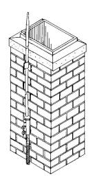
NO. 88-A COMPLETE HEAVY DUTY, CHIMNEY AIR TERMINAL WITH A 1/2" X 4'0" LEAD COATED COPPER AIR TERMINAL. ASSEMBLY INCLUDES SET SCREW, VERTICAL POINT BASE, AND LEAD COATED COPPER PINCH TYPE POINT SUPPORT, BOTH OF WHICH ARE MOUNTED WITH STAINLESS STEEL BOLTS AND LEAD EXPANSION ANCHORS. AIR TERMINAL MUST EXTEND 2'0" MAXIMUM ABOVE CHIMNEY TOP
