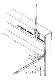
NO. 690X-A PREMIUM DIE CAST POINT BASE FOR SIDE MOUNTING AT PARAPETS OR SCREEN WALLS, ETC. THE PREMIUM DIE CAST CLAMP IS FOR USE WITH ADAPTER TYPE AIR TERMINALS AND CABLES THROUGH NO. 506. MOUNTING HOLES ARE 1<sub>4</sub>" CLEARANCE. ORDER FASTENERS SEPARATELY.
