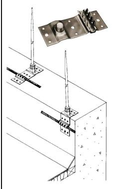
NO. 76-A 2" WIDE COPPER BASE FOR TOP OR FLAT MOUNTING OR AS A FIELD FORMED PARAPET BASE WITH CABLE RUN AT THE INSIDE OF THE PARAPET WALL. BASE INCLUDES A CAST CRIMP TYPE CLAMP FOR CABLES THROUGH NO. 506. POINT STUD ACCEPTS ALL ADAPTER TYPE AIR TERMINALS.
