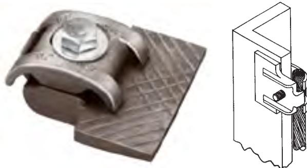
**NO. 142HD**—A LARGER VERSION OF OUR STANDARD FLAT METAL BONDING CLAMP WHICH EXCEEDS THE 3 SQUARE INCH CONTACT AREA REQUIRED FOR MAIN SIZE BONDING CONNECTIONS. CAPACITY IS FOR UP TO 3/8” THICK METAL AND CABLES THROUGH NO. 507.
