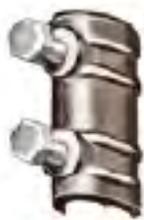
**NO. 230**—A HEAVY DUTY  $2\frac{3}{8}$ " LONG CAST BRONZE TWO BOLT GROUND ROD CLAMP FOR  $\frac{1}{2}$ " GROUND RODS. THIS CLAMP HAS TWO  $\frac{5}{16}$ " STAINLESS STEEL SET SCREWS AND WILL ACCEPT MAIN SIZE CABLES THROUGH NO. 506. THIS CLAMP IS ALSO USED IN SOME CASES TO CONNECT CABLES TO  $\frac{1}{2}$ " AIR TERMINALS OR THROUGH ROOF RISERS, ETC.
