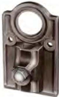
**NO. 703**—A PREMIUM DIE CAST BRONZE BONDING PLATE SIMILAR TO THE NO. 639 BUT WITH A HOLE TO ENGAGE BOLTS OF UP TO 1” IN DIAMETER. CAN ALSO BE FURNISHED WITH A SMALLER BOLT HOLE. THE VISE GRIP CABLE CONNECTION WITH 2” OF CONTACT IS FOR CABLES THROUGH NO. 506. TYPICALLY USED AT COLUMN OR POLE BASE PLATE ANCHOR BOLTS.
