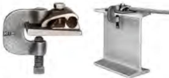
**NO. 701X**—A HEAVY DUTY FORGED STEEL “C” CLAMP WITH BRONZE BONDING PLATE FOR CABLES THROUGH NO. 506 TO STRUCTURAL STEEL PURLINS, CHANNEL IRON, “I” BEAMS, OR ANGLE IRONS. HAS A PREMIUM DIE CAST BOLT PRESSURE TYPE CABLE CLAMP. FITS STRUCTURAL STEEL UP TO 1” THICKNESS AND HAS 9 SQUARE INCHES OF BONDING SURFACE.
