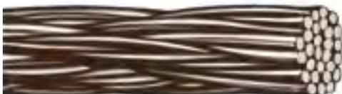
**NO. 507 SUPREME**—28 STRANDS OF .0865" DIAMETER COPPER WIRE,  $\frac{5}{8}$ " DIAMETER, ROPE LAY, 211,500 CIRCULAR MILS, NET WEIGHT 660 LBS. PER 1000 FT.
