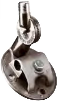
**NO. 30**—THIS PREMIUM DIE CAST BRONZE BASE INCLUDES A SWIVEL ADAPTER SO THAT POINTS MAY BE SET PERPENDICULAR ON A SLOPING ROOF. THE PREMIUM DIE CAST BOLT PRESSURE CONNECTION ACCEPTS CABLES THROUGH NO. 506. MOUNTING HOLES ARE 1/4" CLEARANCE. ORDER FASTENERS SEPARATELY.
