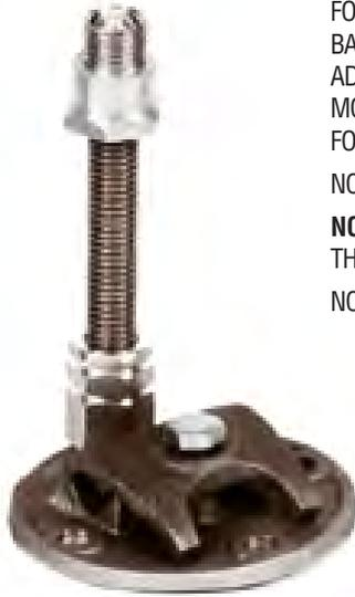
**NO. 709B**—A CONCEALED BASE AND RISER ASSEMBLY FOR METAL OR CONCRETE DECK CONSTRUCTION. RISER BAR IS 1/2" DIAMETER BY 12". TOP ASSEMBLY FITS ALL ADAPTER TYPE AIR TERMINALS. THE PREMIUM DIE CAST MOUNTING BASE HAS A BOLT PRESSURE CABLE CLAMP FOR CABLES THROUGH NO. 506.
