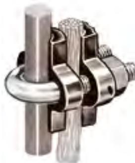
**NO. 430B-A** U-BOLT PARALLEL CLAMP OF CAST BRONZE USED FOR A PARALLEL CONNECTION FROM EITHER ONE OR TWO CABLES OR RODS THROUGH 5/8" DIAMETER TO ANOTHER CABLE OR ROD. U-BOLT, NUTS, AND WASHERS ARE STAINLESS STEEL.
