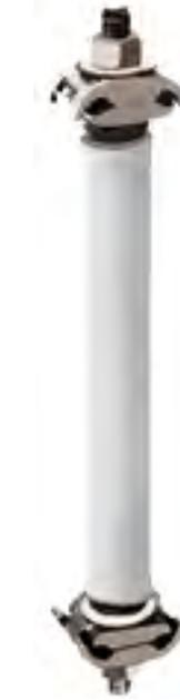
**NO. 156P-4 (-12) OR (-18) OR (-24)**—THIS THROUGH ROOF ASSEMBLY IS SIMILAR TO THE UNIT ABOVE EXCEPT THE RISER PASSES THROUGH THE ROOF DECK WITH THE DOWNLEAD TERMINATION BELOW THE ROOF. FOR CABLES THROUGH NO. 506.
