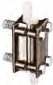
**NO. 604**—AN OVERLAY TYPE GROUND TEST DISCONNECTOR FOR USE ON MASONRY WALLS. COMES COMPLETE WITH BOLTS AND ANCHORS FOR MOUNTING. MADE OF BRONZE FOR USE WITH COPPER CABLES THROUGH NO. 506.
