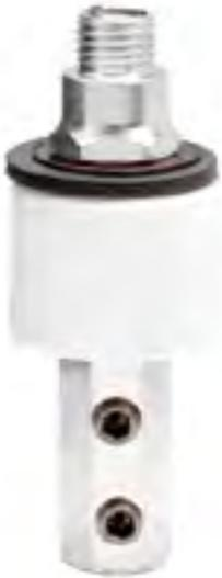
**NO. 155AT**—A THROUGH ROOF BASE WHICH ALLOWS FOR THE INSTALLATION OF A COMPLETE CONCEALED AIR TERMINAL BY ONE TECHNICIAN FROM ABOVE THE ROOF. THIS BASE REQUIRES AN ADEQUATELY SUPPORTED 1" PVC CONDUIT SLEEVE THROUGH THE ROOF. ROOF SEAL IS ACHIEVED VIA AN EPDM SEAL AND SOLVENT WELDED PVC PIPE CAP. IDEAL FOR USE WHERE AIR TERMINALS ARE CONNECTED DIRECTLY TO BUILDING STEEL. FOR CABLES THROUGH NO. 506.
