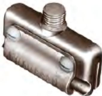
**NO. 691**—A CLAMP TYPE POINT BASE FOR FASTENING TO STANDING SEAM METAL ROOFS WITHOUT THE USE OF MECHANICAL FASTENERS. BOLT PRESSURE CLAMP ACCEPTS CABLES THROUGH NO. 506. EXTERNAL STUD ACCEPTS ALL ADAPTER TYPE AIR TERMINALS.
