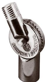
**NO. 27**—A HINGED SWIVEL CONNECTOR DESIGNED SO THAT A POINT MAY BE SET PERPENDICULAR ON A SLOPING ROOF. THE LOWER SECTION FITS ALL BASES WITH EXTERNAL STUDS AND THE UPPER SECTION FITS ALL ADAPTER TYPE POINTS. STAINLESS STEEL SET SCREWS ASSURE A PERMANENT LOCK BETWEEN THE POINT AND THE BASE.
