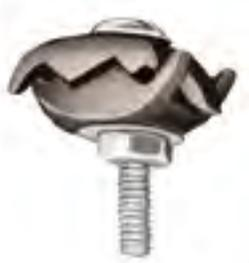
**NO. 143**—A SMALL SIZE PREMIUM DIE CAST PARALLEL CLAMP OF CAST BRONZE WITH 1" OF CONTACT. CLAMPS SECONDARY SIZE TO STANDARD CABLES OR ROUND METAL OBJECTS THROUGH  $\frac{5}{8}$ " DIAMETER.
