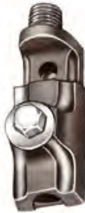
**NO. 690**—A VERTICAL POINT BASE FOR CONNECTION BETWEEN ADAPTER TYPE POINTS AND CABLE THROUGH NO. 506. CONNECTOR HAS MOUNTING HOLE FOR EITHER 1/4" BOLTS OR SCREWS WHICH SHOULD BE ORDERED SEPARATELY. THE CABLE CLAMP IS OF PREMIUM DIE CAST CONSTRUCTION.
