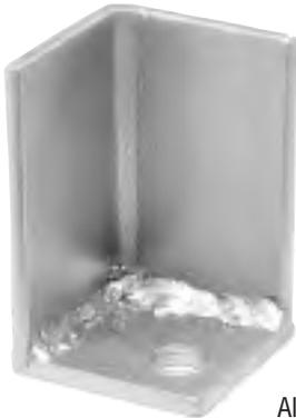
**NO. AT-1B**—A GALVANIZED STEEL "ICE BREAKER" FITTING USED WITH CONCEALED THROUGH ROOF AIR TERMINALS AT THE RAKE EDGE AND EAVE LINES OF METAL ROOF BUILDINGS TO HELP MINIMIZE THE POTENTIAL OF DAMAGE TO THESE AIR TERMINALS FROM SLIDING SNOW AND ICE.
