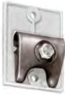
**NO. 702**—A PREMIUM DIE CAST BRONZE BONDING PLATE WITH 8 SQUARE INCH BIMETAL PLATED CONTACT AREA. THE PRESSURE TYPE CABLE CONNECTOR IS FOR CONDUCTORS THROUGH NO. 506. THIS PLATE WILL ACCOMMODATE EITHER A “DEAD-END” OR CONTINUOUS THROUGH CABLE ROUTE. THE TWO HOLES WILL FIT EITHER SHEET METAL SCREWS OR ¼” MACHINE SCREWS.
