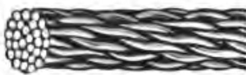
**NO. A37 BEN FRANKLIN**—37 STRANDS OF 13 GAUGE ALUMINUM WIRE, 9/16" DIAMETER, SMOOTH CONCENTRIC TWIST, 192,000 CIRCULAR MILS, NET WEIGHT 190 LBS. PER 1000 FT.
