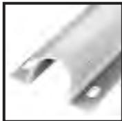
**NO. 242XP**—AN 8'0" MOLDED PVC GUARD (LIGHT GREY COLOR) FOR PROTECTION OF EXPOSED DOWN CONDUCTORS. GUARD CAN BE MOUNTED TO WOOD, METAL OR MASONRY SURFACES. SIX FASTENERS ARE RECOMMENDED AND SHOULD BE ORDERED SEPARATELY. MOUNTING HOLES ARE FOR 1/8" MAXIMUM DIAMETER FASTENERS.
