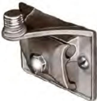
**NO. 678LA**—A HEAVY DUTY RIGHT ANGLE PARAPET BASE WITH AN EXTERNAL STUD FOR ALL ADAPTER TYPE POINTS. THIS BASE IS DESIGNED FOR MOUNTING NEAR THE TOP OF THE WALL FOR USE WITH 12"-24" POINTS WHICH WILL REQUIRE NO FURTHER SUPPORT. THE POINT IS HELD OUT FROM THE WALL TO CLEAR A COPING OVERHANG OF UP TO 1 1/2". PREMIUM DIE CAST BOLT PRESSURE CABLE CLAMP ACCEPTS CABLES THROUGH NO. 506.
