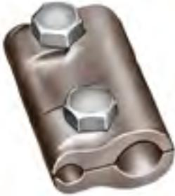
**NO. 565**—A CAST BRONZE 2" LONG PARALLEL CLAMP FOR CONNECTING MAIN SIZE CABLES THROUGH NO. 506 TO SECONDARY SIZE NO. 14X THROUGH NO. 509 CABLE OR WIRE. SPECIFY CABLE SIZE COMBINATION.
