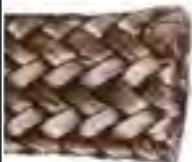
**NO. 503**—AN EXTRA FLEXIBLE FLAT CONDUCTOR, 480 STRANDS OF 30 GAUGE COPPER WIRE,  $\frac{3}{4}$ " WIDE, 48,250 CIRCULAR MILS, NET WEIGHT 159 LBS. PER 1000 FT. THIS CONDUCTOR IS USED TO FIELD FABRICATE FLEXIBLE JUMPERS OF LONGER LENGTH USING STANDARD CLAMPS/LUGS FOR TERMINATIONS.
