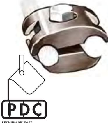
**NO. 141**—A PREMIUM DIE CAST BRONZE CLAMP WITH 1 1/2" OF CONTACT TO CONNECT ALL MAIN SIZE CABLES THROUGH NO. 506 TO ALL ROUND METALLIC BODIES THROUGH 5/8" DIAMETER.
