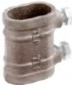
**NO. 519**—A LARGE, HEAVY DUTY  $3\frac{7}{8}$ " LONG CAST BRONZE GROUND ROD CLAMP FOR  $\frac{3}{4}$ " GROUND RODS. THIS CLAMP HAS TWO  $\frac{5}{16}$ " STAINLESS STEEL SET SCREWS AND WILL ACCEPT CABLES THROUGH NO. 507.
