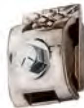
**NO. 142**—A PREMIUM DIE CAST BRONZE BONDING CLAMP WITH  $1\frac{1}{2}$ " OF CONTACT TO CONNECT ALL CABLES THROUGH NO. 506 TO FLAT METALLIC BODIES SUCH AS CHANNEL IRONS, FLASHINGS, ANGLE IRONS, ETC. PRIMARILY TO SERVE AS A CABLE HOLDER ON "I" BEAMS, ANGLE IRONS, ETC. FITS MAXIMUM THICKNESS OF  $\frac{5}{8}$ ".
