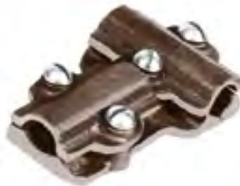
**NO. 706X-A** HEAVY DUTY, DOUBLE CAP TEE SPLICER OF CAST BRONZE FOR NO. 507 AND 250MCM CABLES. EACH CABLE IS SECURED BY A PRESSURE TYPE CLAMP WITH 2" OF CONTACT LENGTH.
