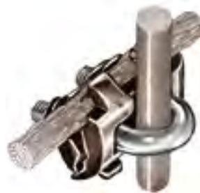
**NO. 493**—THIS  $\frac{5}{16}$ " STAINLESS STEEL U-BOLT TYPE ROD TO CABLE CLAMP IS A VERY VERSATILE CONNECTOR FOR CLAMPING ALL MAIN SIZE CABLES FROM NO. 29X THROUGH NO. 507 TO GROUND RODS THROUGH  $\frac{3}{4}$ " DIAMETER. THIS CLAMP CAN ALSO BE USED TO CONNECT AIR TERMINALS, RISER BARS, REINFORCING RODS, AND SMALL PIPING (THROUGH  $\frac{7}{8}$ " DIAMETER) TO CABLES.
