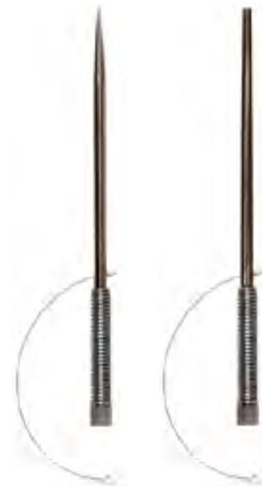
**NO. 55SP**-FLEXIBLE AIR TERMINALS FOR USE WHERE WINDOW WASHING OR OTHER MOVABLE EQUIPMENT CONFLICTS WITH FIXED AIR TERMINAL. ADAPTER FITS ALL EXTERNAL STUD TYPE BASES. SOLID POINT PORTION IS 1/2" DIAMETER COPPER WITH NICKEL PLATED TIP. OVERALL HEIGHT IS 12". THE HEAVY STAINLESS STEEL SPRING PROVIDES A 90° TILT IN ANY DIRECTION. COMES COMPLETE WITH A STAINLESS STEEL SAFETY TIE-OFF CABLE WITH LUG FOR ATTACHING TO BOLT AT BASE.
