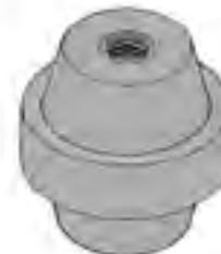
**NO. 38316**—A RED 600 VOLT STAND-OFF INSULATOR WITH 1 1/2" FACE DIAMETER AND 2" HEIGHT. INSERTS ARE THREADED 3/8"-16.
