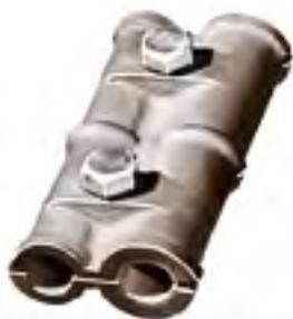
**NO. 744-A** HEAVY DUTY 3 1/2" LONG BIMETAL PARALLEL CLAMP USED AS A BIMETALLIC CONNECTOR FOR JOINING ALUMINUM AND COPPER CABLES NO. 32 THROUGH NO. 506 TO NO. A24 THROUGH NO. A37 ALUMINUM CABLES.
