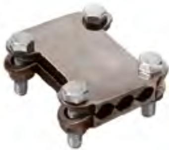
**NO. 607-A** 3 GROOVE PARALLEL CLAMP WHICH CAN BE USED TO CONNECT TWO CABLES THROUGH NO. 506 TO A 1/2" ROD, POINT, OR ANOTHER CABLE.
