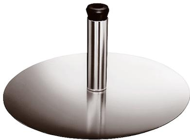
**NO. 746M**—A PURE COPPER THROUGH ROOF FLASHING THAT HAS AN 8" DIAMETER BASE WITH A 7/8" DIAMETER X 8" TALL COPPER TUBE. COMES WITH EPDM RUBBER SEAL.
