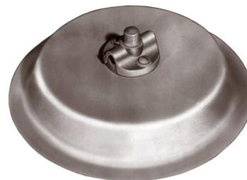
**NO. 694**—THIS PAN TYPE POINT BASE IS FOR FLAT ROOFS. INCLUDES A COMBINATION POINT TO CABLE BASE CONNECTOR WITH EXTERNAL STUD FOR ALL ADAPTER TYPE POINTS. ACCEPTS CABLES THROUGH NO. 506. THE PAN IS FILLED WITH CEMENT ON THE JOB AND IS INVERTED AFTER THE CEMENT SETS. NO. 589 PAN-TYPE CABLE SUPPORTS ARE USED IN CONJUNCTION WITH THIS BASE. CAN BE USED WITH OR WITHOUT ADHESIVE. OVERALL WEIGHT HOLDS BASE AND CABLE SUPPORTS IN PLACE.
