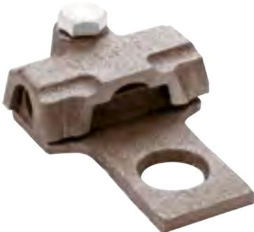
**NO. 706RDC**—A COMBINATION CABLE SUPPORT AND BONDING CLAMP WITH A  $\frac{5}{8}$ " CLEARANCE HOLE. DEVELOPED FOR USE ON BOLTED STRUCTURES SUCH AS RADOMES, METAL STRUCTURE COVERS, AND CABLE TRAYS, ETC., WHERE STRUCTURAL BOLTS SERVE TO MOUNT THIS FITTING. PRESSURE CAP CONNECTOR ALLOWS FOR CONTINUOUS CABLE ROUTE. FOR CABLES THROUGH NO. 506.
