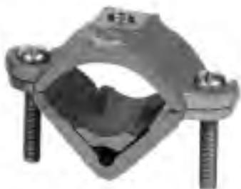
**NO. 240P-3**—A BIMETAL PLATED, CLAMP TYPE AIR TERMINAL BASE FOR MOUNTING ON PIPES, ROUND HANDRAILS, ETC. UP TO 1¼" O.D. HAS INTERNAL THREAD FOR 3/8" LESS ADAPTER TYPE POINTS. (CLASS I ONLY.)
