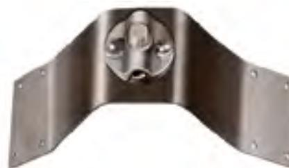
**NO. 532**—A HEAVY DUTY 3/4" WIDE, COPPER RAISED RIDGE SADDLE. BENDS TO FIT ANY ROOF SLOPE AND HOLDS POINT AND CABLE SLIGHTLY ABOVE THE CENTER OF THE RIDGE. PRESSURE TYPE CABLE CLAMP IS FOR CABLES THROUGH NO. 506. STUD ENGAGES ALL ADAPTER TYPE POINTS. (USE NO. 533 ATTACHMENT TO HOLD AND SUPPORT THE CABLE BETWEEN POINT LOCATIONS.)
