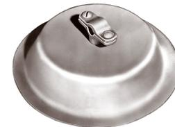
**NO. 589**—AN ALL COPPER PAN TYPE CABLE SUPPORT FOR FLAT ROOFS. PAN IS FILLED WITH CEMENT ON THE JOB AND INVERTED AFTER THE CEMENT SETS. THE WEIGHT OF THIS UNIT HOLDS THE ATTACHMENT IN PLACE. CABLE SUPPORT ACCEPTS ALL CONDUCTORS THROUGH NO. 506.
