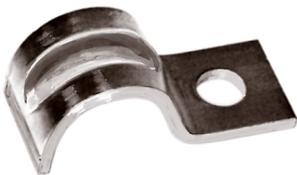
**NO. 168M**—A HEAVY DUTY STAMPED COPPER ONE HOLE CLIP FOR NO. 507 CABLE OR 5/8" TUBE WITH 1/4" HOLE. ORDER FASTENERS SEPARATELY.
