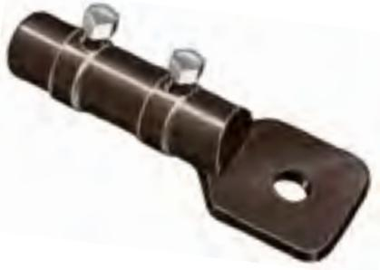
**NO. 551**—A HEAVY DUTY BRONZE BONDING LUG THAT HAS TWO STAINLESS STEEL SET SCREWS FOR BONDING ALL STANDARD CABLES THROUGH NO. 506 TO FLAT METAL SURFACES. BOLT HOLE SIZE IS NORMALLY  $\frac{3}{8}$ " BUT LARGER HOLES CAN BE FURNISHED WHEN SPECIFIED.
