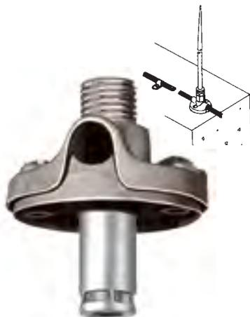
**NO. 78**—A ONE BOLT BRONZE BASE WITH PRESSURE TYPE CABLE CONNECTION FOR INSTALLATION ON FLAT MASONRY. COMPLETE WITH STAINLESS STEEL MACHINE SCREW AND 5/16" PAK-TITE ANCHOR. STUD ENGAGES ALL ADAPTER TYPE POINTS. ACCEPTS CABLES THROUGH NO. 506.
