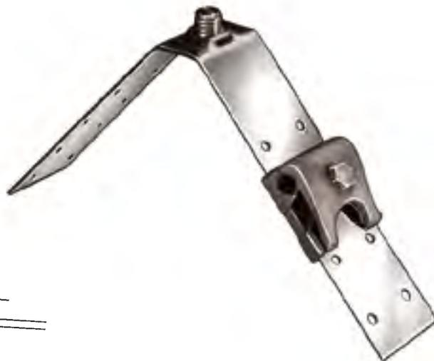
**NO. 71X**—AN ADJUSTABLE RIDGE SADDLE OF PURE COPPER, 2" WIDE X 15" LONG, THAT CAN BE FORMED FOR ANY ROOF SLOPE. THE PREMIUM DIE CAST CABLE CLAMP IS FOR CABLES THROUGH NO. 506. THE 5/8" EXTERNAL STUD IS FOR ALL ADAPTER TYPE POINTS.
