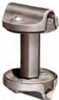
**NO. 740**—A CABLE TO CABLE WALL OUTLET FOR IMBEDDING IN CONCRETE TO PROVIDE A CONNECTION BETWEEN A CABLE CONCEALED IN A WALL OR FLOOR TO AN EXTERIOR CABLE. MADE OF BRONZE AND FITS ALL CABLES THROUGH NO. 506.
